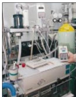
Addition of nitric oxide to inspired gas in a mechanical ventilator. Inspired concentration of nitric oxide and expired concentration of nitrogen dioxide must be measured
